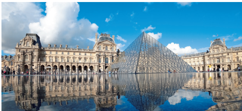
Photocatalysis acts as an antifouling and antifogging effect simply by the irradiation of light. It has also been used in the glass covering the pyramid-shaped entrance of the Louvre Museum. The glass maintains its transparent beauty by decomposing dirt.
