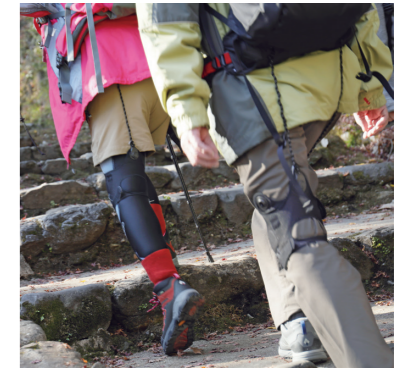
Participants of a sightseeing tour wearing the Himico, a powered exoskeleton that supports walking.
