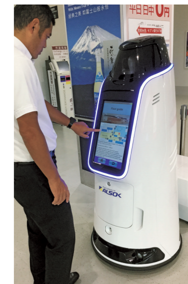
The REBORG-Z with a large built-in display. It can also display emergency evacuation advice in multiple languages during a disaster.
