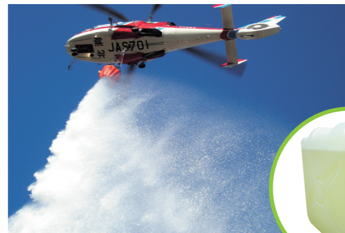
Top: The Fire Department of Kitakyushu, a city designated as a SDGs Future City in Japan, is proactively using the eco-friendly foam to fight fires. Right: A soap-based fire-fighting foam formulated from naturally-sourced soaps, made solely from vegetable fats and potassium hydroxide.
