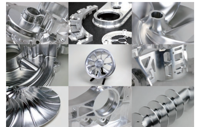
Prototypes cut from aluminum. Digitalizing fabrication processes allows HILLTOP to quickly adjust to customer requests and remake items.
