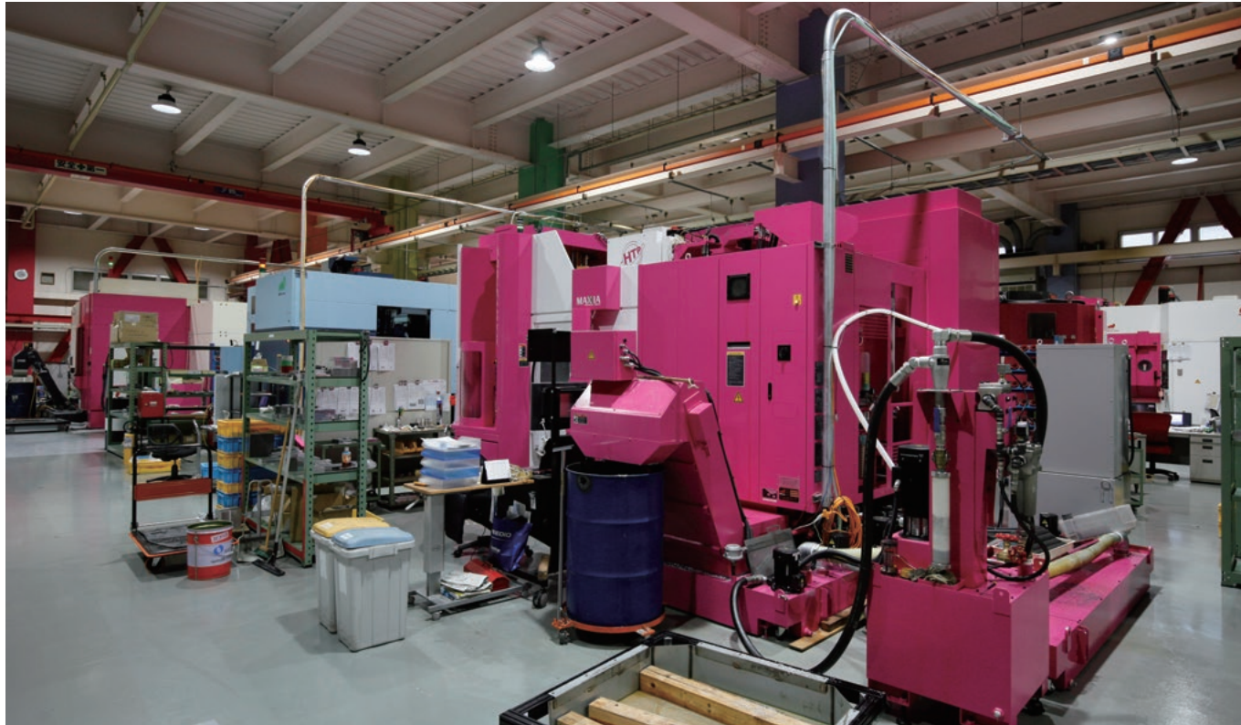
Processing machines with HILLTOP's trademark pink color scheme are arranged in neat lines inside a factory. Most operations are automated and require little human intervention.
