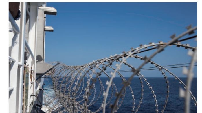
As measures against crimes at sea, protection measures such as shielding the vessel with barbed wire making it harder to board can prove effective. Providing such advice is one of the activities performed by ReCAAP ISC. © Perspectives / Getty Images
