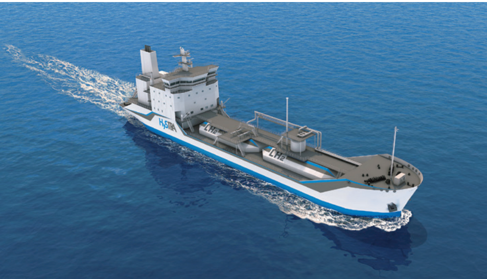
CG image of the world's first liquefied hydrogen carrier that will be used by the project led by HySTRA**. In the future, even these hydrogen carrying ships will run on hydrogen.
