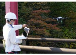
Drones are expected to play an active part in inspecting and surveying bridges, dams, wind power plants, and other sites that are hard to access by humans, as well as in assessing the situation at the time of a disaster. The picture depicts a bridge-survey experiment.
