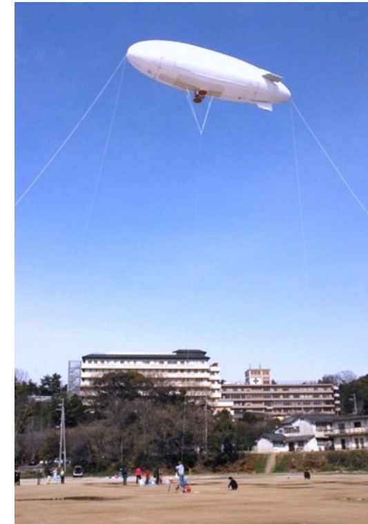
The photo shows a microwave wireless power-transfer experiment from an airship to the ground, conducted by Kyoto University in 2009. Due to its ability to send and receive power over longer distances than other contactless power-transfer methods, the technology to wirelessly transmit power with microwaves shows promise for use in a variety of applications on the ground, such as supplying power to disaster areas where infrastructure has been disrupted. SHINOHARA LAB., KYOTO UNIV.
