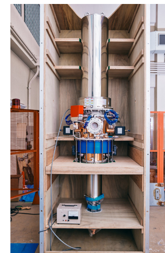
A gyrottron, a special machine that heats the plasma fuel with microwaves to 100 million degrees Celsius or higher. It operates in a similar way to an extremely powerful microwave oven.
