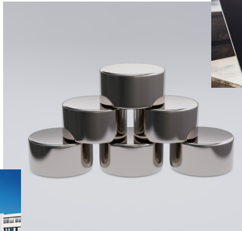
Neodymium magnets (center) are mainly composed of iron—an abundantly available and inexpensive substance—along with neodymium and boron. Their low cost has led to their rapid popularization and has greatly improved performance for a wide range of products: from air conditioners to personal computers, electric vehicles, and wind turbines. AFLO (top left photo); SHUTTERSTOCK (center, top right, and bottom left); EYEEM (bottom right)
