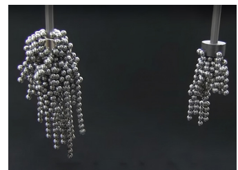
A major feature of the neodymium magnet (left) is its strong magnetic force; it is about 10 times stronger than a ferrite magnet (right), the most widely used magnet in the world, including for daily necessities. NATIONAL INSTITUTE FOR MATERIALS SCIENCE
