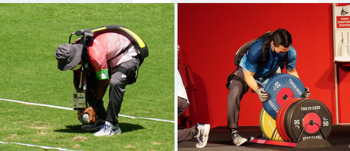
Power Assist Suits reduced back stress and helped officials pick up shots at shot-put venues, while also aiding personnel in the exchange of weight plates during powerlifting competitions. TOKYO 2020
