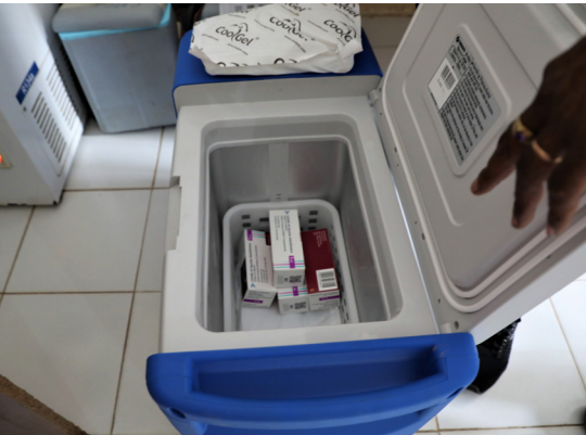
Vaccine transport boxes developed by Twinbird Corporation are among the equipment provided by Japan. Since the boxes can draw power from a car's cigarette-lighter socket and are resistant to shaking, they are already being used in Timor-Leste to store and transport vaccines in areas where the power supply is unstable. JICA
