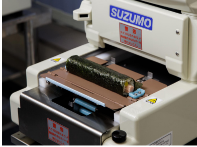
Suzumo Machinery's robots can produce perfect sushi rolls in an instant, a tricky task (right). Becoming more popular in recent years, such rice-serving machines also dish out rice in pre-measured quantities, helping to save on food.
