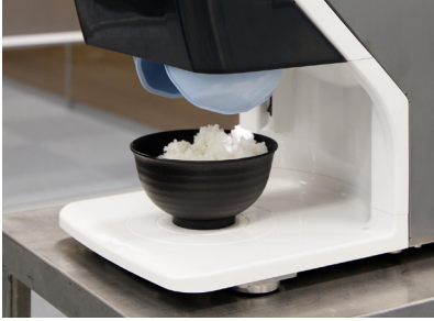
Suzumo Machinery's robots can produce perfect sushi rolls in an instant, a tricky task (right). Becoming more popular in recent years, such rice-serving machines also dish out rice in pre-measured quantities, helping to save on food.
