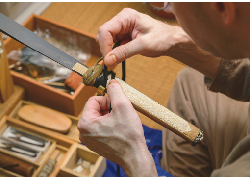
The process called tsukamaki (hilt wrapping) involves wrapping leather cord around the hilt to strengthen it and provide a better grip. The diamond-patterned tsukamaki is so solidly wrapped that it must have been indestructible on the battlefield.
