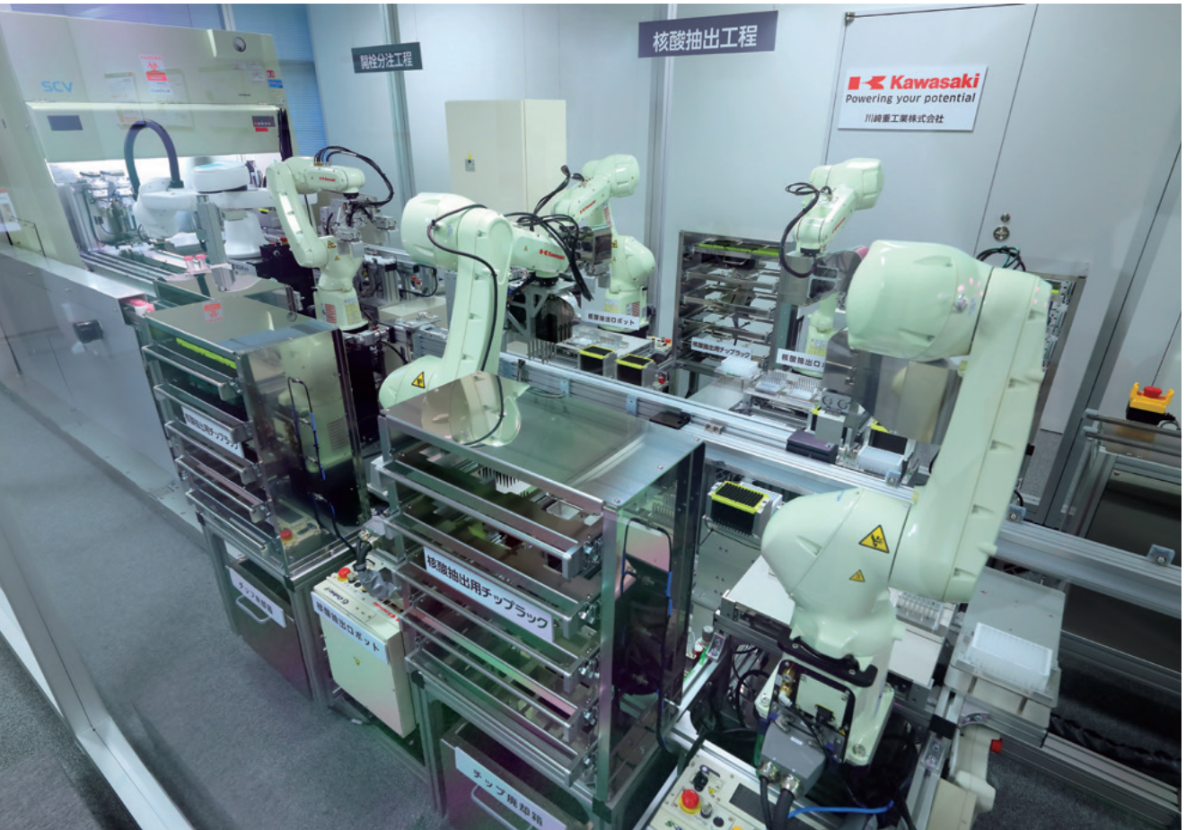
Top: Robots conduct every step of the PCR testing process, protecting healthcare workers from the risk of infection. Right: The technical capabilities cultivated in the development of industrial robots enable such actions as opening a lid with a mechanical arm.
