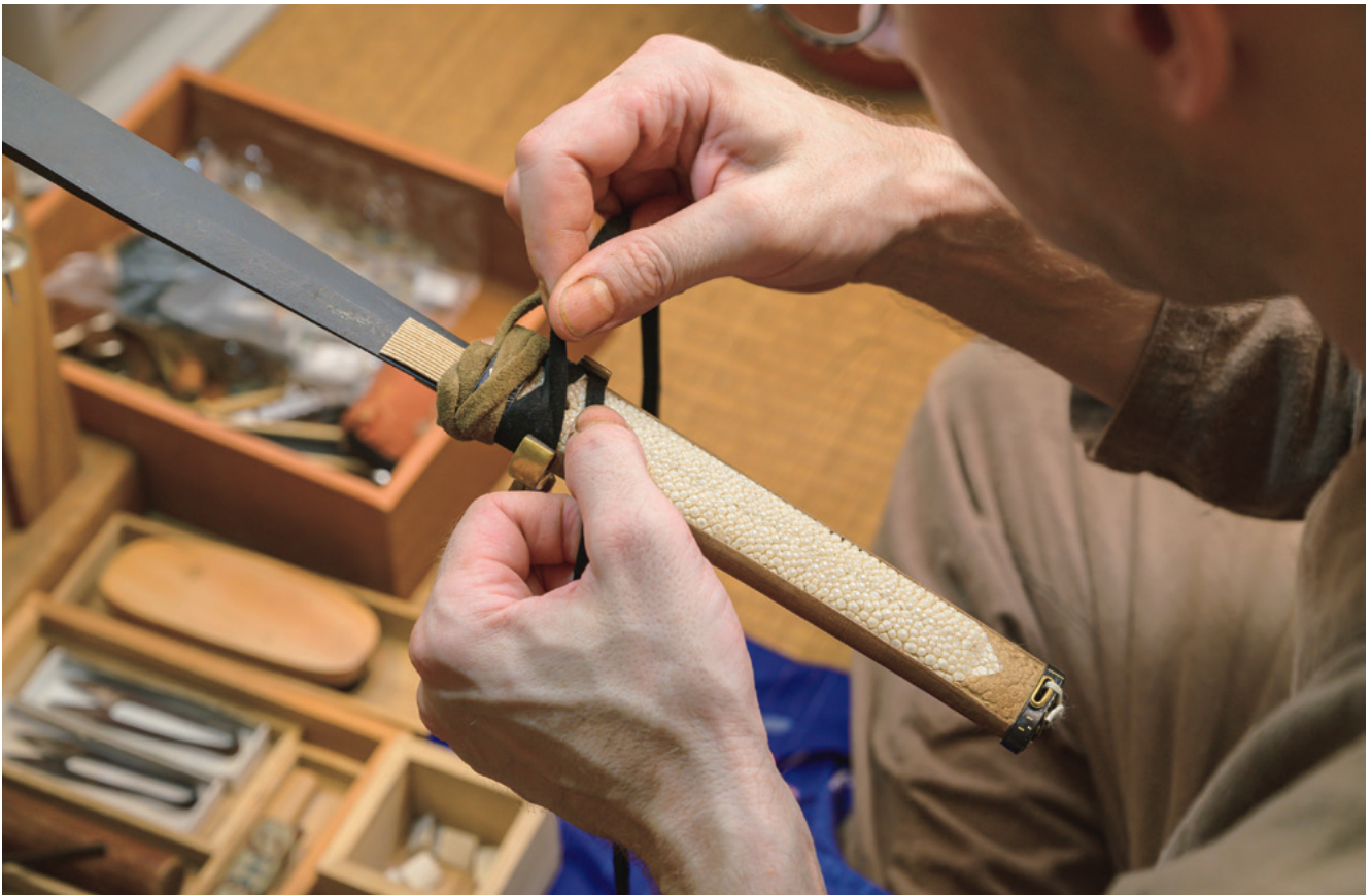
The process called tsukamaki (hilt wrapping) involves wrapping leather cord around the hilt to strengthen it and provide a better grip. The diamond-patterned tsukamaki is so solidly wrapped that it must have been indestructible on the battlefield.
