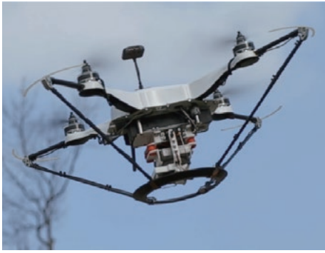
Construction range and soil volume is calculated by combining the drone's measurement data with the completion plan. Based on that data, the construction equipment is semi-automatically controlled.
