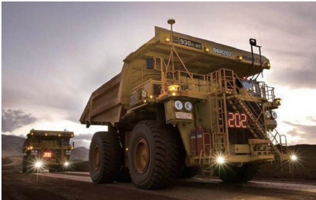
"AHS" is a system that uses GPS along with a gyroscope for detecting angle and speed and combines it with technology such as laser guidance to remotely control unmanned super-large dump trucks. The system is in use at the Chuquicamata copper mine in Chile and the Yandicoogina iron mine in Australia.
