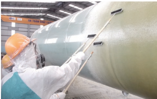
Under Tamada Industries' supervision, FRP is being manually crimped to a tank.
