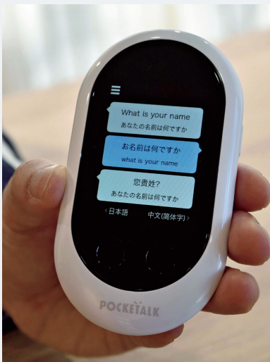
When you speak into the terminal, the spoken content is automatically converted into the language of the other party and is read aloud.
