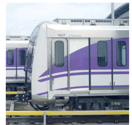
All-stainless steel stock that is robust, light-weight and resistant to corrosion.
