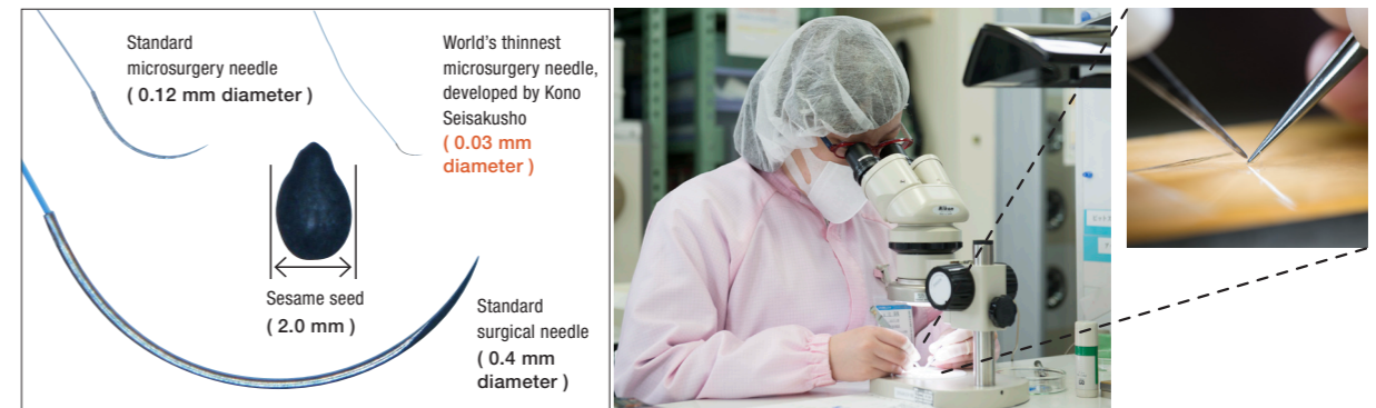
3. A standard surgical needle (bottom) and microsurgery needles from Kono Seisakusho. The tiny size of the latter is evident. 4. Threading a microsurgery needle, barely visible to the naked eye, using a microscope and tweezers. Women are active in many of Kono Seisakusho's operations, including this kind of precision work.
